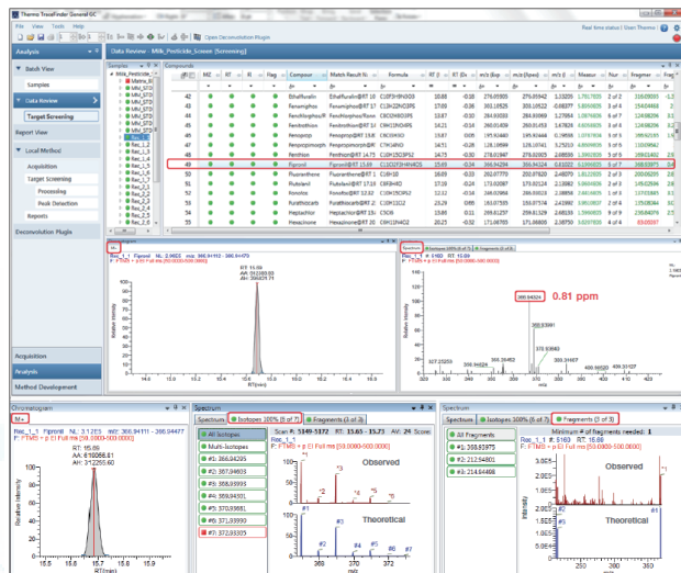
Figure 3. Extracted ion chromatogram along with spectra, isotopic pattern, and fragments for fipronil in the sample spiked at 0.005 mg/kg concentration
