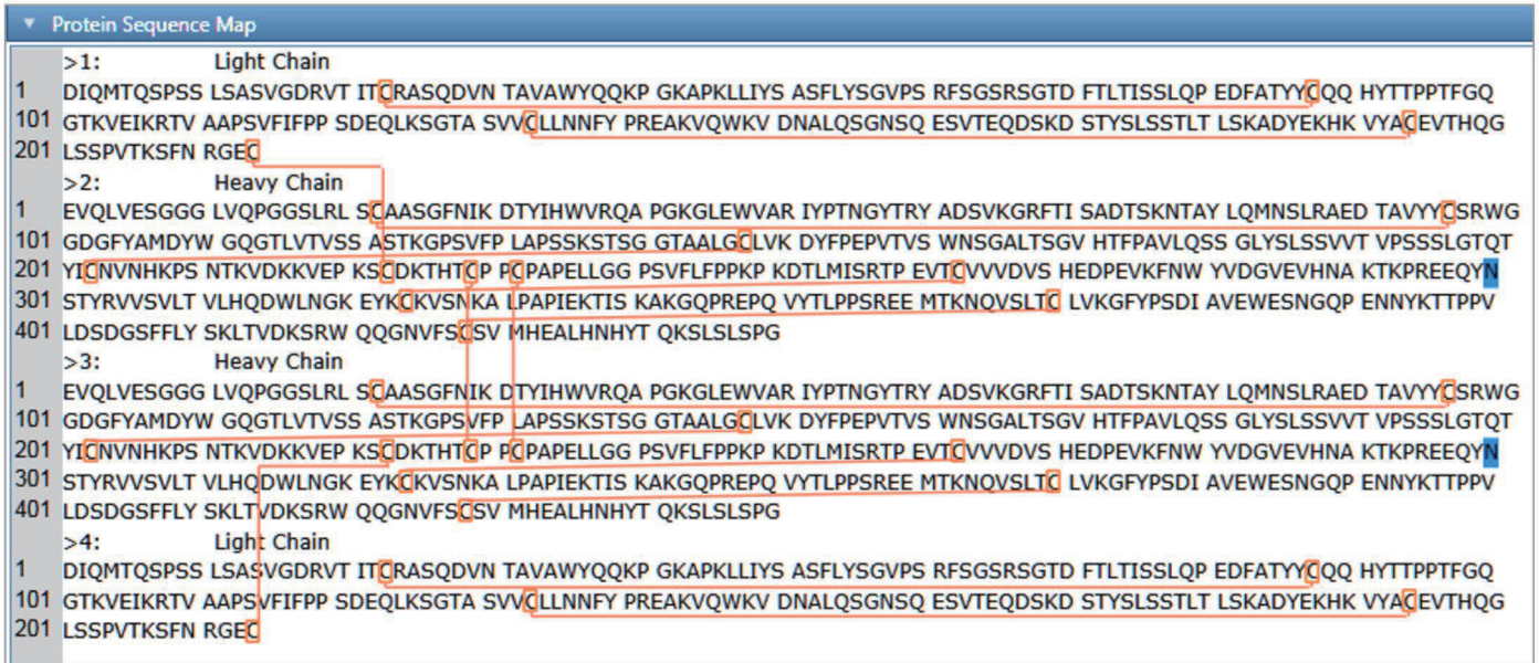
Figure 1. Setting up the Protein Sequence Map for intact protein analysis. For intact mass analysis, trastuzumab amino acid sequence is added as four separate polypeptide chains, with two copies each of light and heavy chains. Disulfide bonds were added by right-clicking at the site of a cysteine residue to create a linkage, then right-clicking at the site of a second cysteine residue to complete the linkage. The blue highlighted asparagine residues are N-glycan consensus sites (Nx[S/T]), which are known to become glycosylated in trastuzumab. A fixed modification at these sites was added by left double-clicking and selecting a specific glycoform for attachment.
