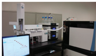
FIGURE 1. HDX work station coupled online to the Orbitrap Fusion mass spectrometer
