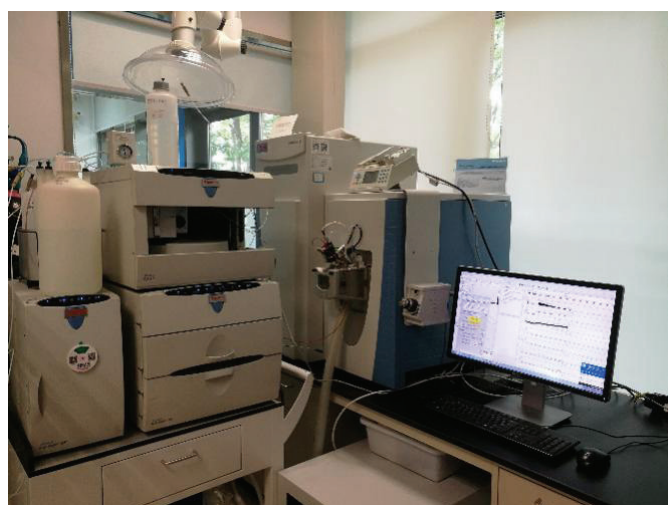
图2. Thermo Scientific Dionex ICS-5000+离子色谱与Q Exactive质谱仪联用实物图
